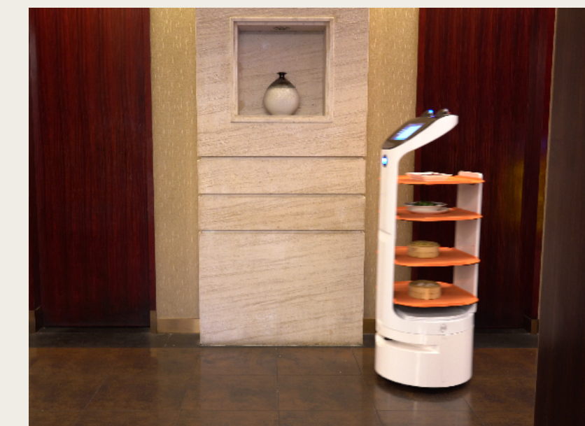
After reaching the target floor, Automatically switch maps and start delivery
